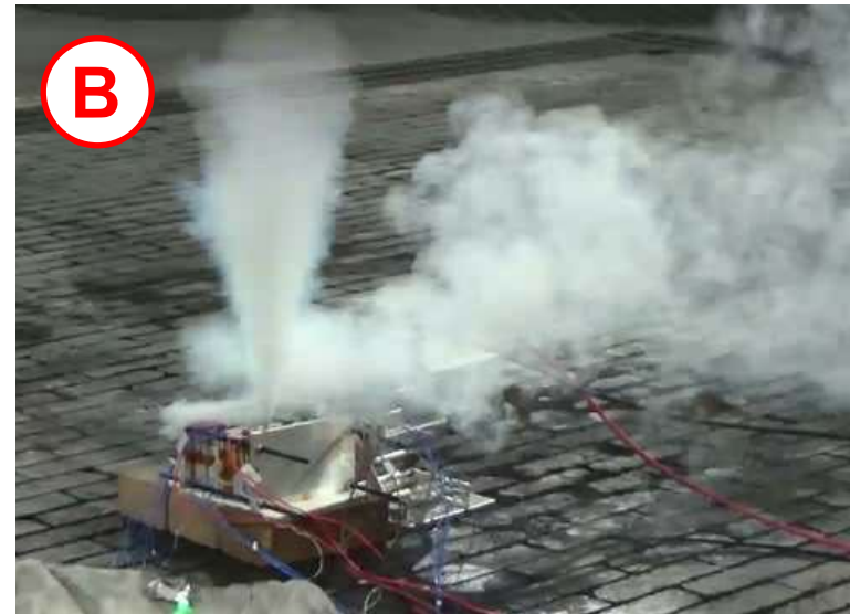
Outset of a cell thermal runaway
